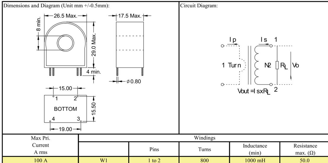
Date applies for one primary turn (single passage of primary wire through toroid hole).
